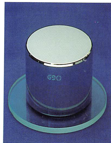
Figure 1.2 The standard platinum-iridium kilogram is kept at the International Bureau of Weights and Measures in Sèvres, France.
