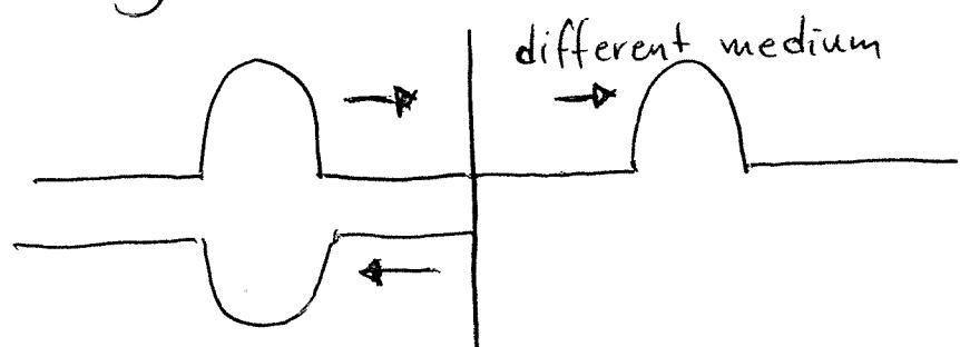
pulse is partially transmitted and partially reflected and partially absorbed
