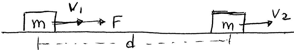
$$\text{Work} = F \cdot d = \frac{1}{2} m v_2^2 - \frac{1}{2} m v_1^2$$
